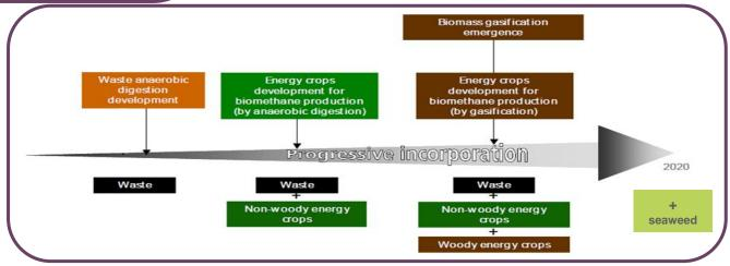
Anaerobic digestion and gasification are complementary processes for the production of green gas/biomethane (different resources and maturity).
